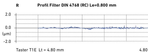
Inner surface roughness measured at a SYGEF Plus T90° equal d250 SDR33 / PN10
