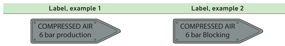
GIV.20 Labelling of compressed air lines (examples)
