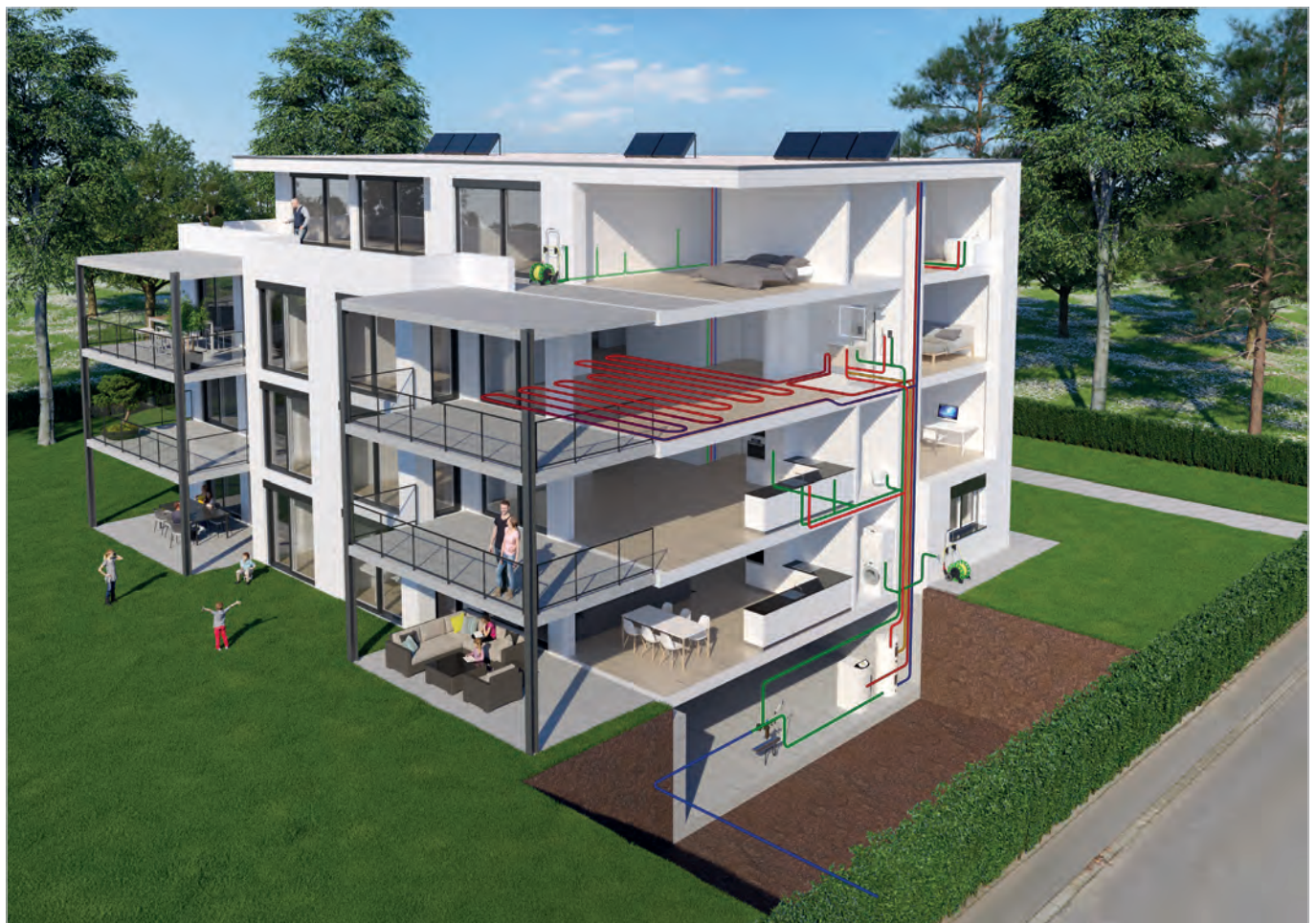
GIV.1 Drinking water installation (exemplary, typical representation)
