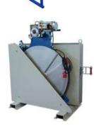
GF 800 Butt fusion machine for construction site
