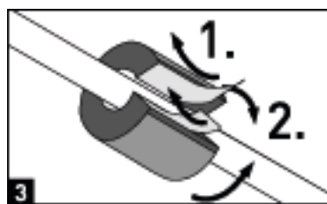
Assemble insulation 1. Peel off foil 2. Press on contact area
