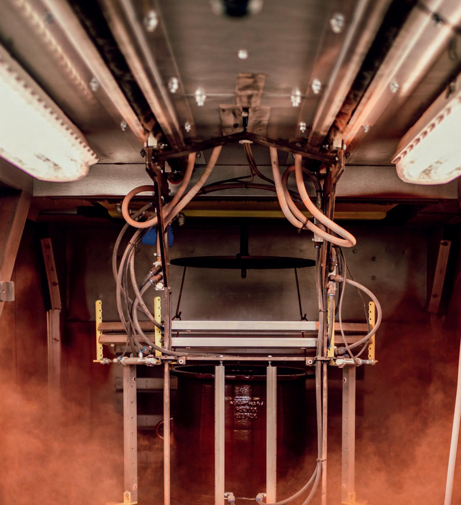
The pre heated ductile cast iron body gets dipped into the Resicoat® Epoxy powder. The heat causes the powder to fusion bond with the ductile cast iron permanently. The coating is GSK approved and 100% safe for drinking water.
