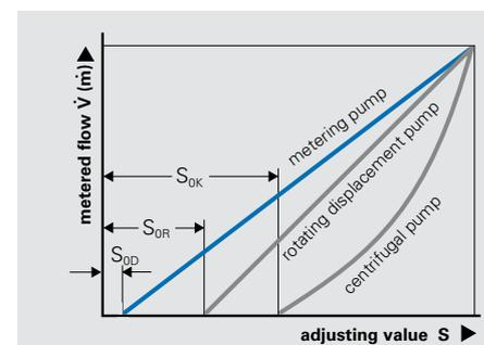
Advantage of the metering pump: the pressure stiff characteristics
