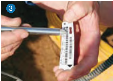
Automatic fusion data input. Easy and fast input of the necessary fusion data with the barcode reader.
