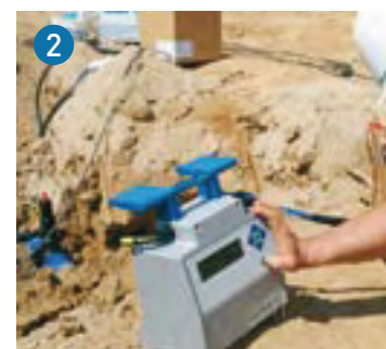
MSA Plus control units. Manual or automatic fusion-data input.
