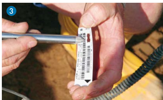
Automatic fusion data input: Easy and fast input of the necessary fusion data with the barcode reader used for example traceability.
